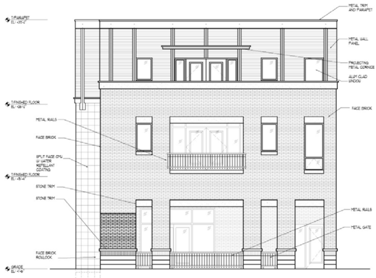
REAR ELEVATION SCALE: 1/4" = 1'-0"
